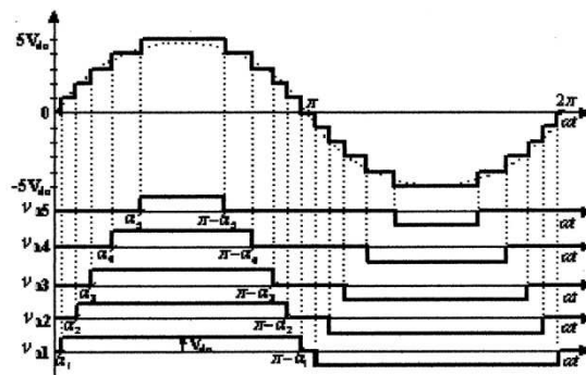
Figure 2: Output Voltage Waveform of an 11-Level Inverter
